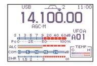
The multi-function meter displays the internal temperature meter for your reference.
